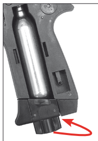
Tighten cylinder retention screw.
